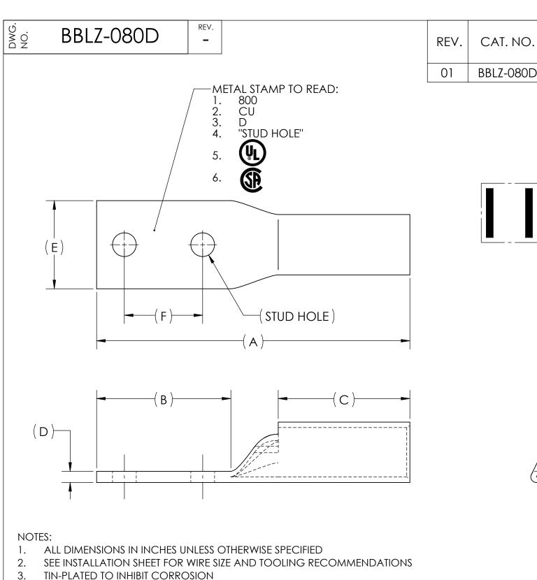
APPROX. **DIMENSIONS** STRIP WEIGHT STUD HOLE LENGTH В С D Ε F Α (LB) 1/2 7.00 3.00 .25 2.94 1.97 1.75 BBLZ-080D 1.027 3.10
