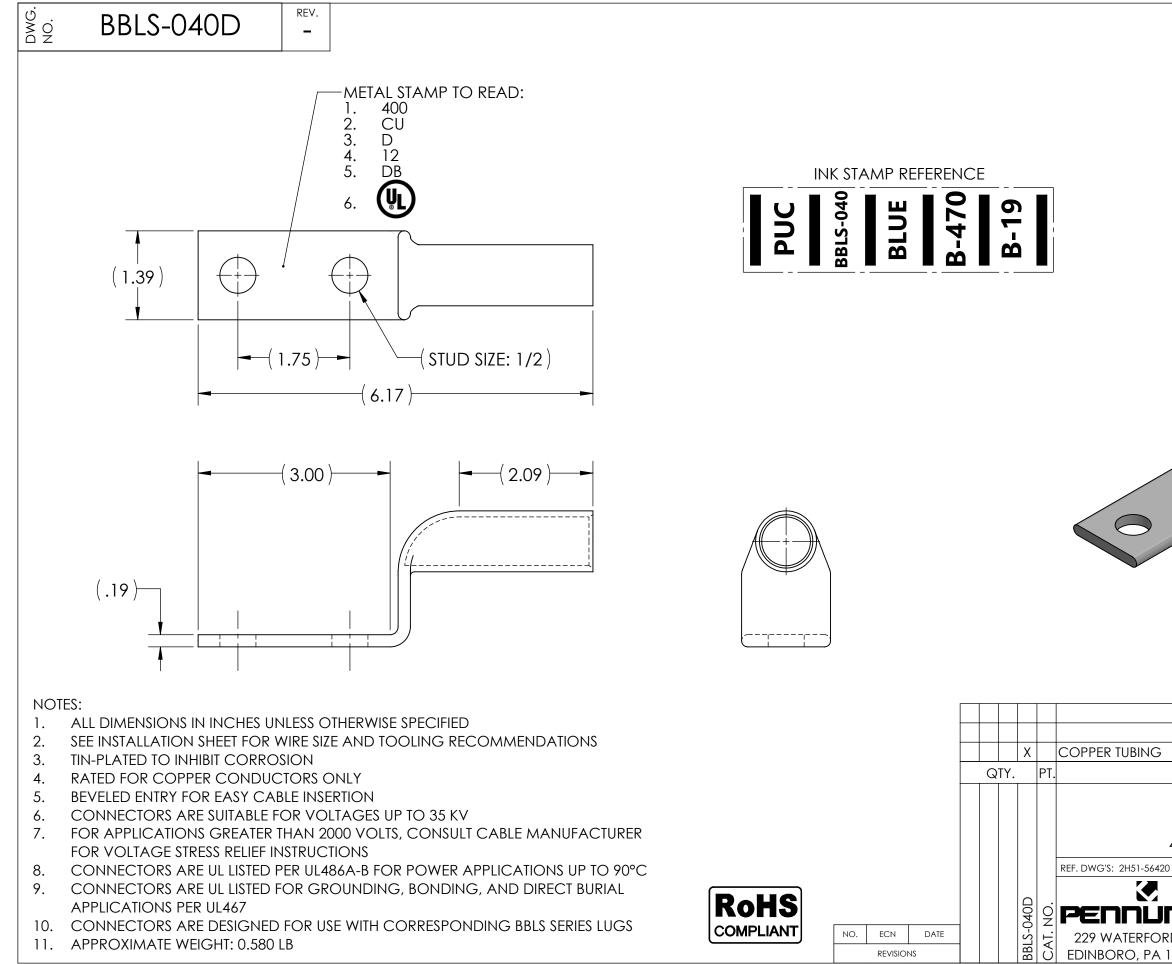
10. CONNECTORS ARE DESIGNED FOR USE WITH CORRESPONDING BBLS SERIES LUGS
