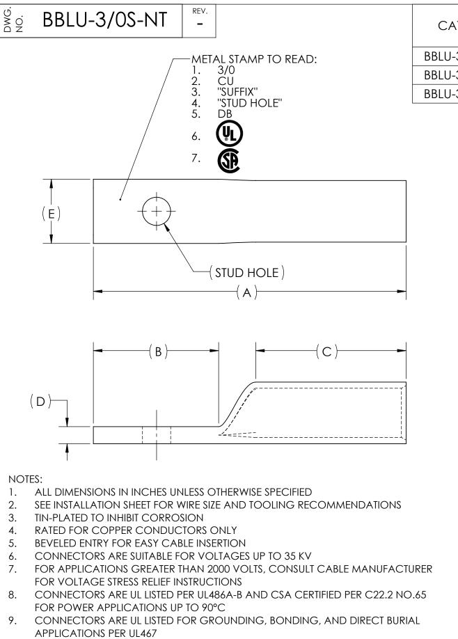
10. CONNECTORS ARE CSA CERTIFIED FOR GROUNDING, BONDING, AND DIRECT BURIAL APPLICATIONS PER C22.2 NO.41
