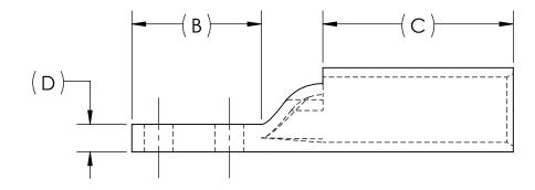
USE BELOW OPTIONAL SUFFIXES FOR ALTERNATE LUG CONFIGURATIONS: -45 FOR 45° BENT PAD -90 FOR 90° BENT PAD
