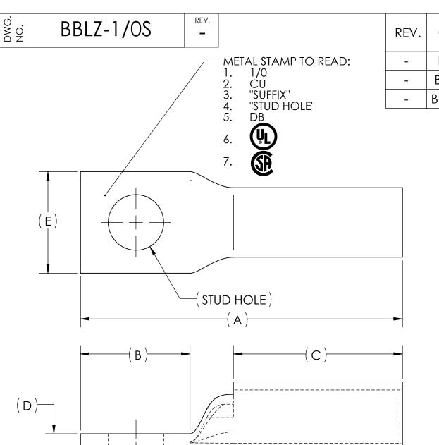
APPROX. **DIMENSIONS STRIP SUFFIX WEIGHT** CAT. NO. STUD HOLE LENGTH В С D Ε Α (LB) BBLZ-1/OS .75 1.34 .73 S 5/16 2.44 .13 0.065 1.50 **S**2 2.38 1.25 3/8 .81 .13 .75 0.062 1.38 BBLZ-1/0S2 3.06 1.38 1.38 BBLZ-1/0S15 \$15 1/2 .13 .75 0.079 1.50
