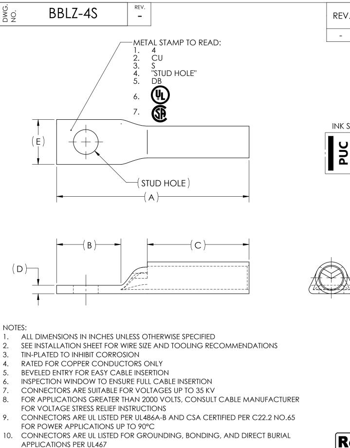
11. CONNECTORS ARE CSA CERTIFIED FOR GROUNDING, BONDING, AND DIRECT BURIAL APPLICATIONS PER C22.2 NO.41
