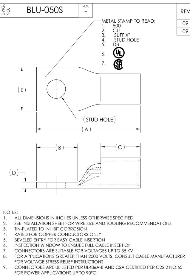
10. CONNECTORS ARE UL LISTED FOR GROUNDING, BONDING, AND DIRECT BURI. **APPLICATIONS PER UL467**
