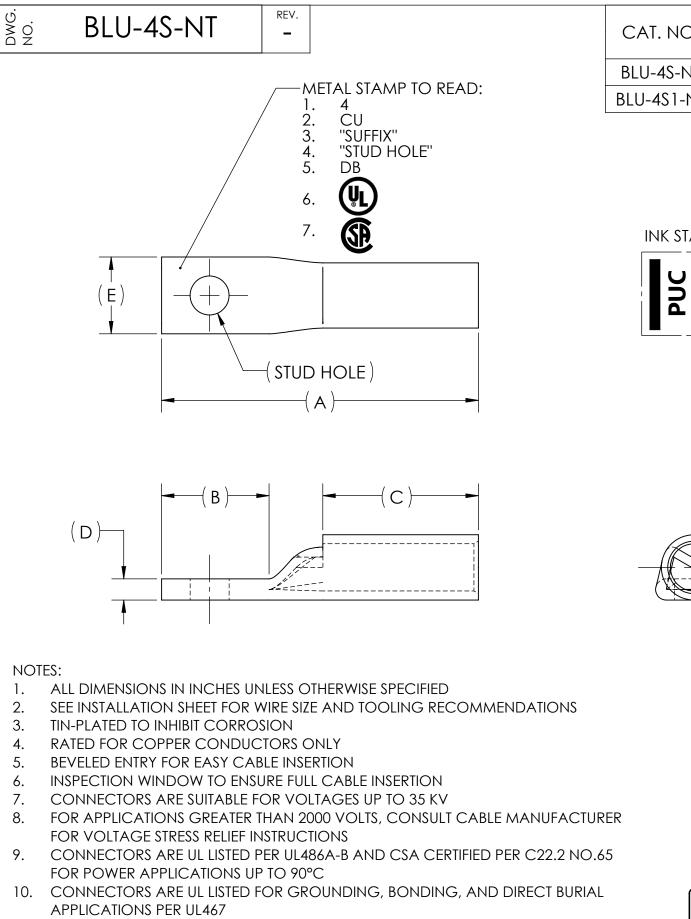
11. CONNECTORS ARE CSA CERTIFIED FOR GROUNDING, BONDING, AND DIRECT APPLICATIONS PER C22.2 NO.41
