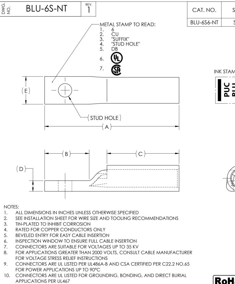
11. CONNECTORS ARE CSA CERTIFIED FOR GROUNDING, BONDING, AND DIRECT APPLICATIONS PER C22.2 NO.41
