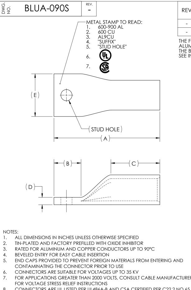
8. CONNECTORS ARE UL LISTED PER UL486A-B AND CSA CERTIFIED PER C22.2 N FOR POWER APPLICATIONS UP TO 90°C
